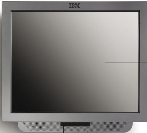
IR touchscreen display has no plastic film to scratch and is designed to help avoid the need for recalibration
